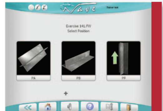
Selection of parameters such as welding position
