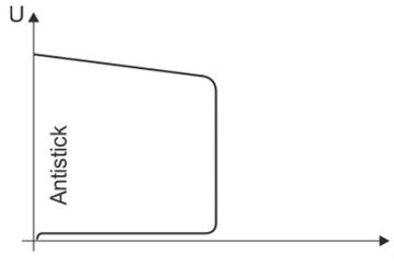
**The Antistick feature prevents the electrode from annealing.** Should the electrode stick despite the Arcforce feature, the machine automatically switches to the minimum current within approx. one second. This prevents the electrode from annealing. Check the welding current setting and correct for the welding task in hand.
