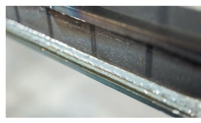
The welding result from the innovative EWM forceArc puls welding process is excellent: high quality, deep penetration and hardly any straightening and finishing work is needed.
