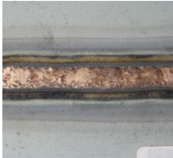
Brazing galvanized sheet metal
