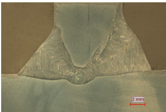
Full penetration, welded on both sides
