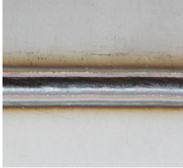
Welding high-alloy sheet metal
