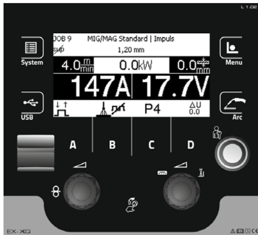
Figure 30: Control of a synergy-programmed MIG/MAG machine (high-tech)
