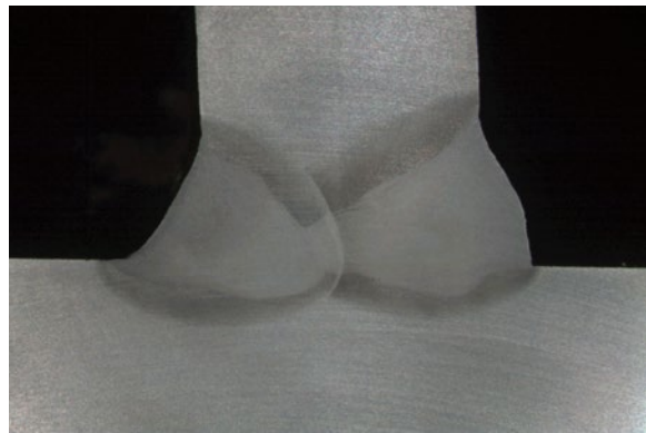
Full penetration, welded on both sides
