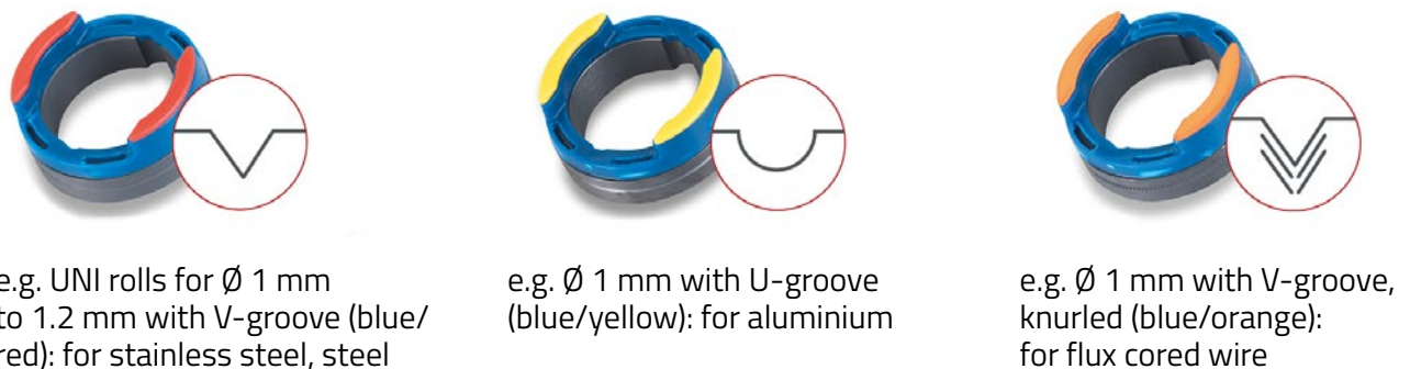
Figure 15: Drive rolls with differing groove geometries
