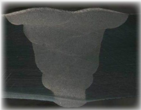
Pass build-up for pipe welding
