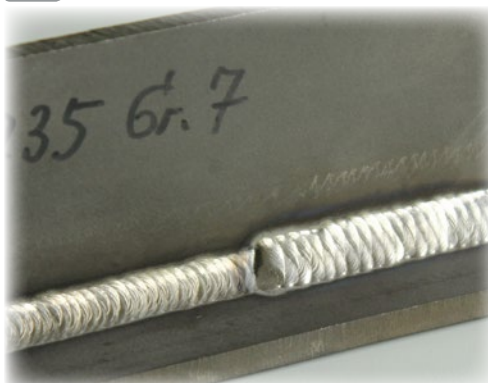
PB Filler and final pass, titanium grade 7 (3.7235)
