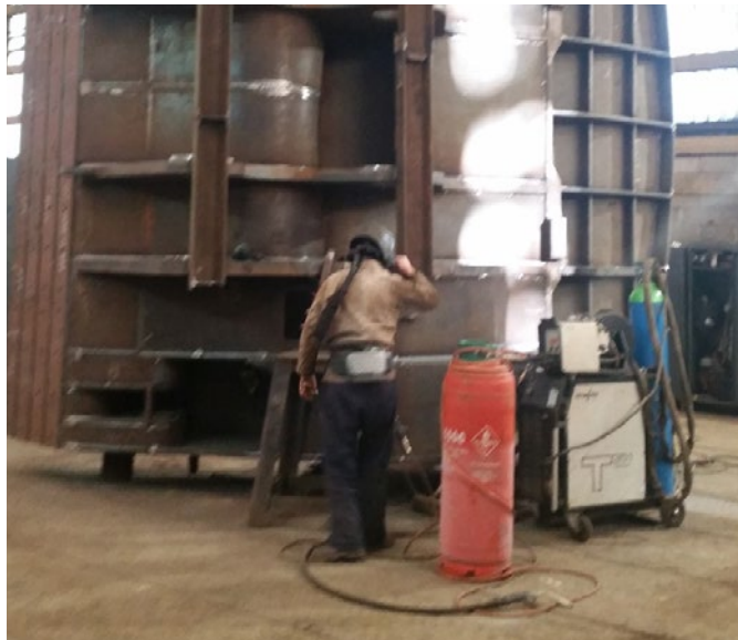
With dimensions of 5,640 x 4,550 x 4,820 mm and a total weight of 70 tonnes, the PC8000 face shovel bucket has a volume of 42 m 3 . It is used to extract oil sand in Canada.
