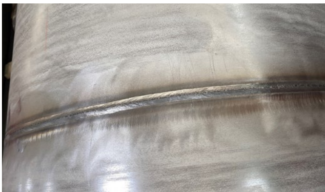
The coldArc pulsed short arc delivers the highest welding quality in the root pass.
