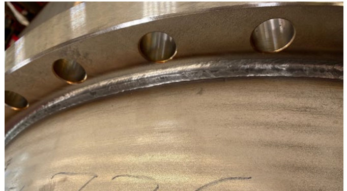
Low-spatter and x-ray proof weld seams can be achieved by choosing the right welding process and characteristics.
