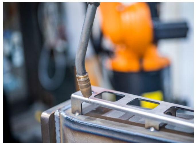
Using the welding torch, the robot detects the exact position of the component put in place. It uses the wire tip of the filler metal as a probe and detects the short circuit. From this, the program derives the exact position of the component.
