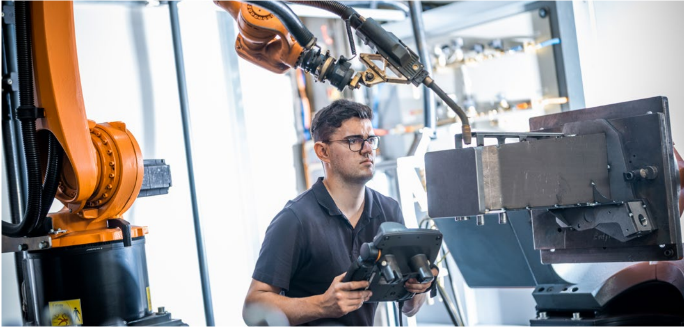
Programmer Lukas Kegel teaches in the welding paths of the component by running the torch along the welding seams and saving the path & welding speed.
