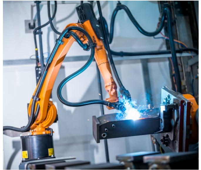
MAG welding the taught-in contour of the preheated fine-grained steel component. The component is clamped in the positioner with a load-bearing capacity of 500 kg.
