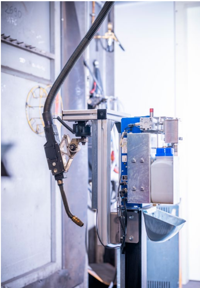
The welding torch in its parking position. The robot can pick up the torch using a pneumatic coupling situated above. The torch cleaning station is located to the right.
