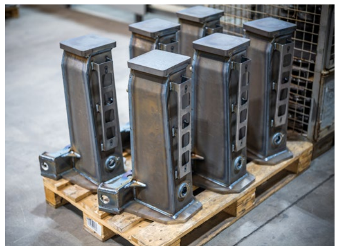
Fully welded booth arms. Manual tack welding of the parts takes 45 minutes, and subsequent welding with the robot (including preheating above and below) takes 35 minutes.
