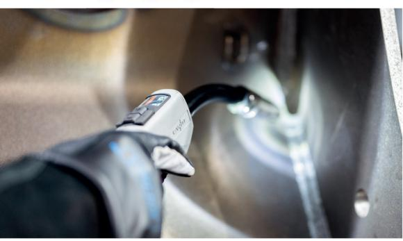
Thanks to the integrated control and graphic display on the RD3X function torch, all the relevant parameters can be set directly on the welding torch. The LED lighting illuminates dark working areas.
