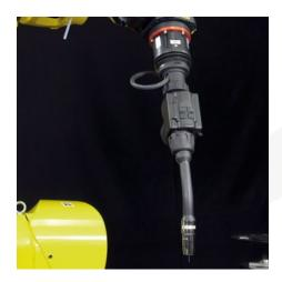
Integrated into the special coldArc<sup>†</sup> XQ robot welding torch is a highly dynamic motor which causes the wire to move back and forth in the high frequency range.
