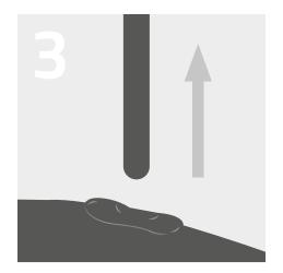
As a result of the active mechanical backward movement, the wire is drawn from the weld pool with high precision and the arc reignites.
