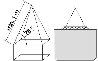
Fig. Lifting principle
