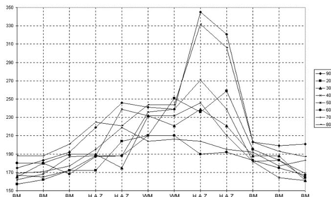
Fig.12, test result hardness course to Vickers (HV5)
