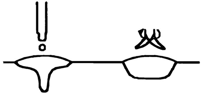
Fig. 3, Penetration profiles of the conventional spray arc (left) and rotary spray arc (right) [2].
