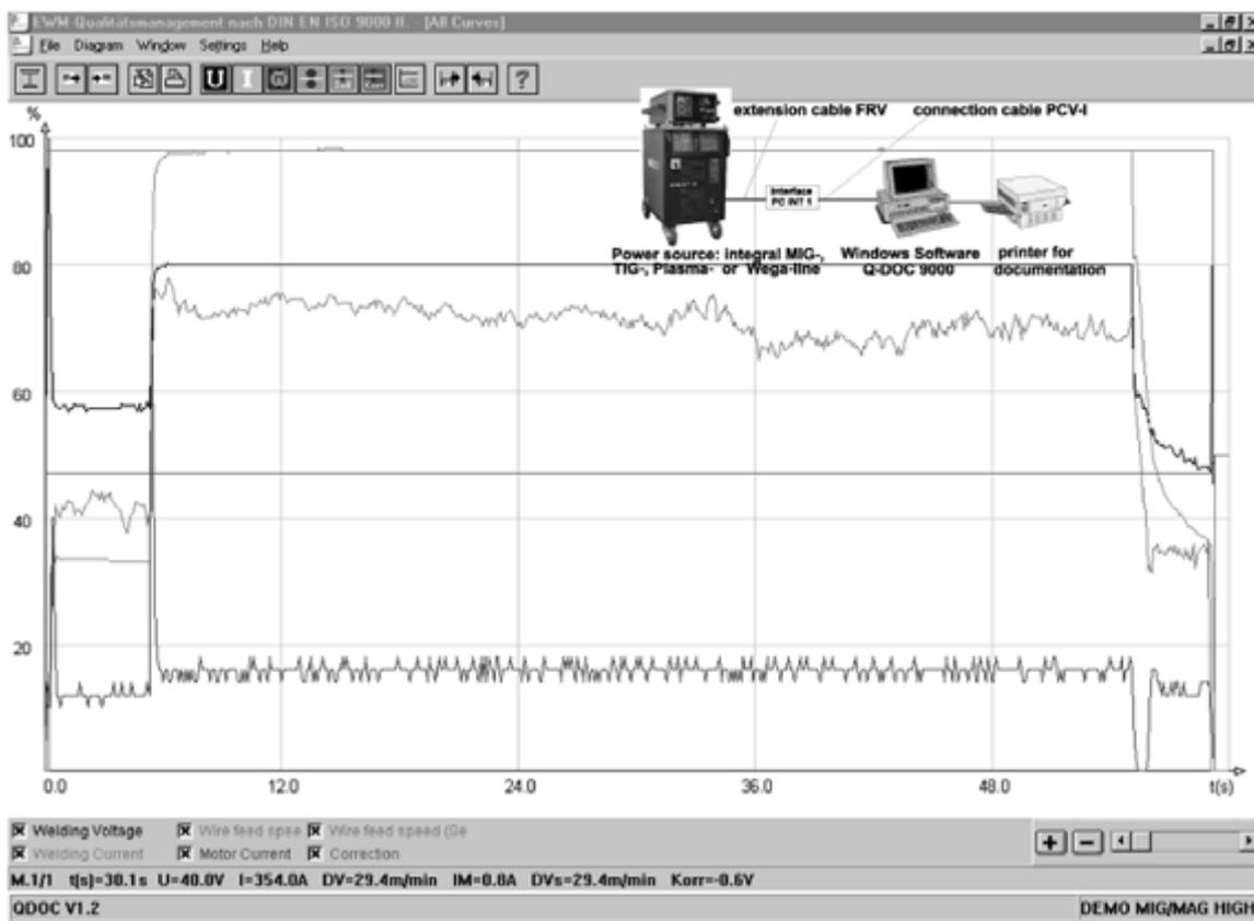
Fig. 8, Graphical representation of the welding parameters with HIGH- SPEED® welding.
