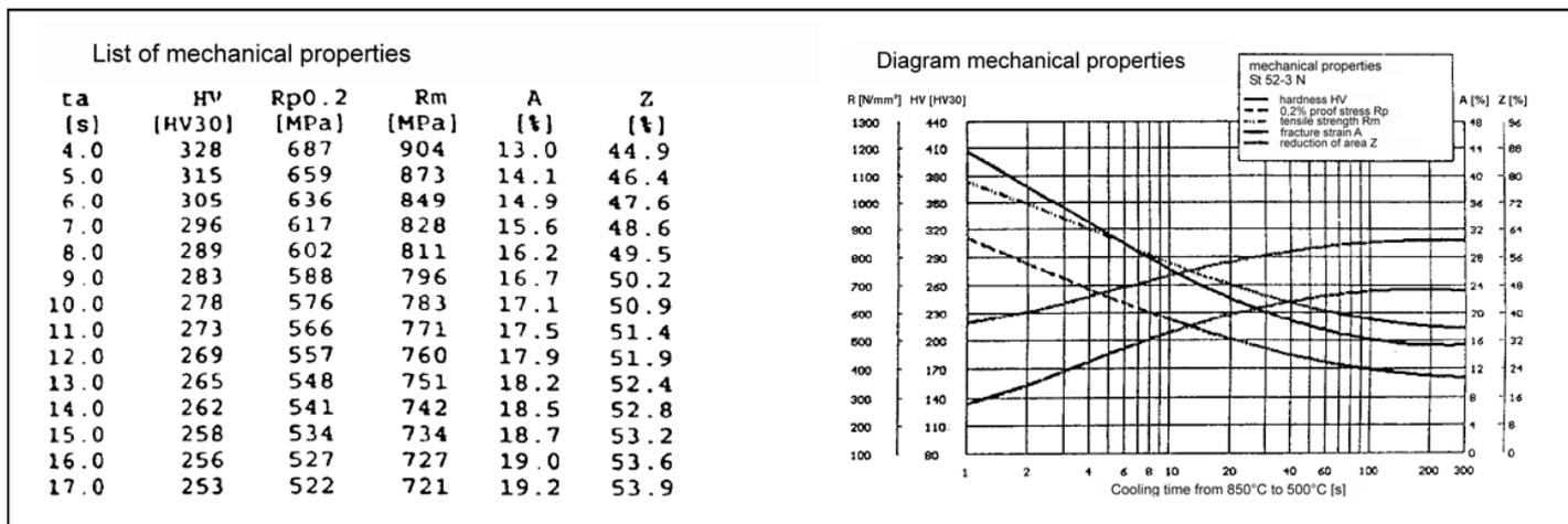
Fig. 13, Mechanical properties of ST 52-3 as a function of cooling time  $t_{8/5}$
