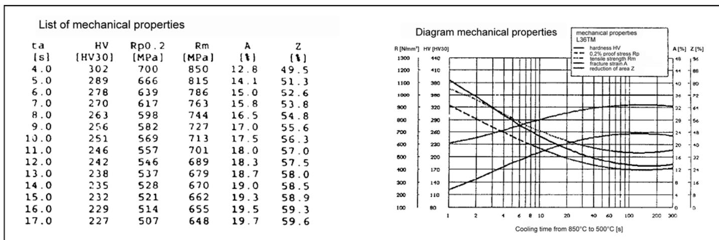
Fig. 14, Mechanical properties of L36TM as a function of cooling time  $t_{8/5}$
