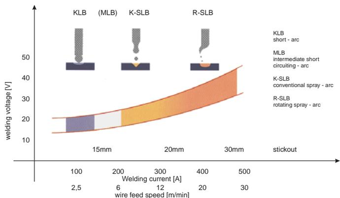
Fig. 4, Types of arc and their power ranges. [2]
