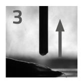
As a result of the active backward movement, the wire is drawn from the weld pool with high precision and the arc reignites.
