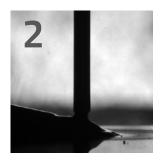
At the moment when the wire comes into contact with the molten metal, the molten droplet in the short circuit is transferred to the weld pool. The RCC module controls the short-circuit resolution.
