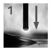
The wire is actively moved toward the weld pool at high speed. The arc ignites on the molten metal and produces a molten droplet at the same time.
