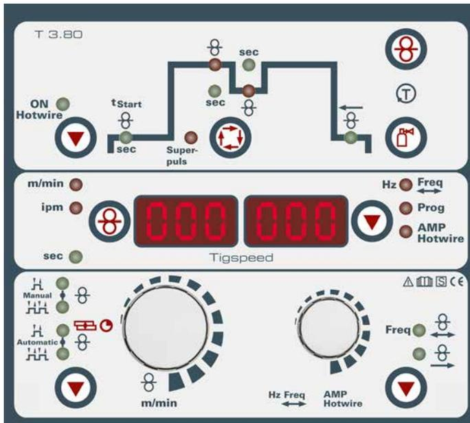
A controller with one-knob operation makes handling really straightforward, and the digital display guarantees reproducible parameter settings.
