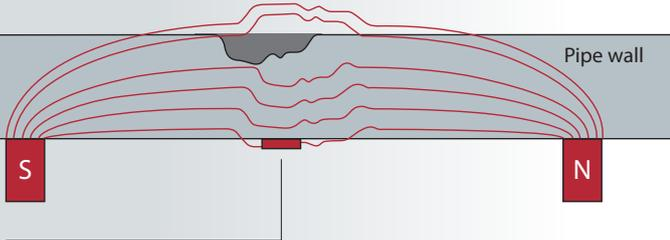
A strong magnetic field is applied parallel to the pipe wall. The magnetic flux lines are deflected if:
