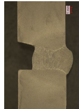
Material thickness 10 mm, one-sided bevel 15 degrees, air gap 4 mm
