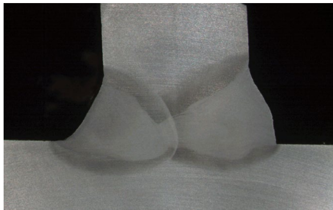
PB Full penetration, welded on both sides
