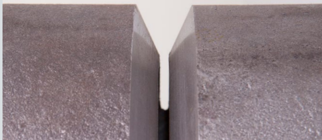
Weld preparation of root welds on pipes, 60° included angle with 3 mm air gap
