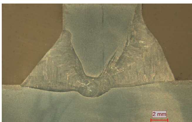
PB Full penetration, welded on both sides
