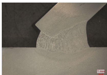
Web plate material thickness 10 mm, included angle 35°
