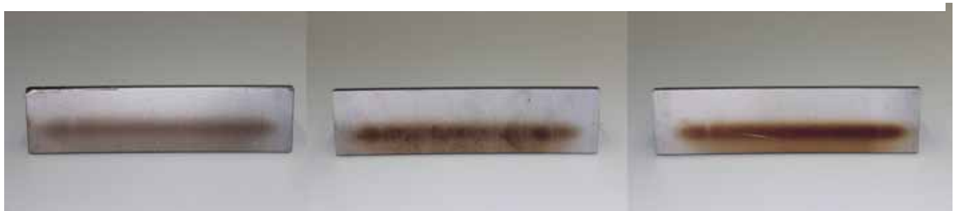
Figure 7: Comparison of the seam appearance and discolouration, plate t = 10 mm, wire speed = 13 m/min; forceArc puls on left, forceArc in centre, pulse on right
