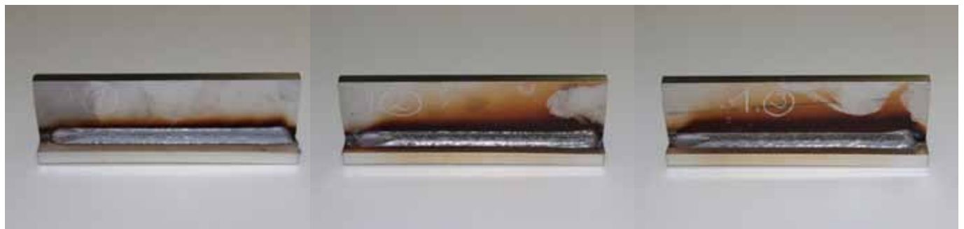
Figure 7: Comparison of the seam appearance and discolouration, plate t = 10 mm, wire speed = 13 m/min; forceArc puls on left, forceArc in centre, pulse on right
