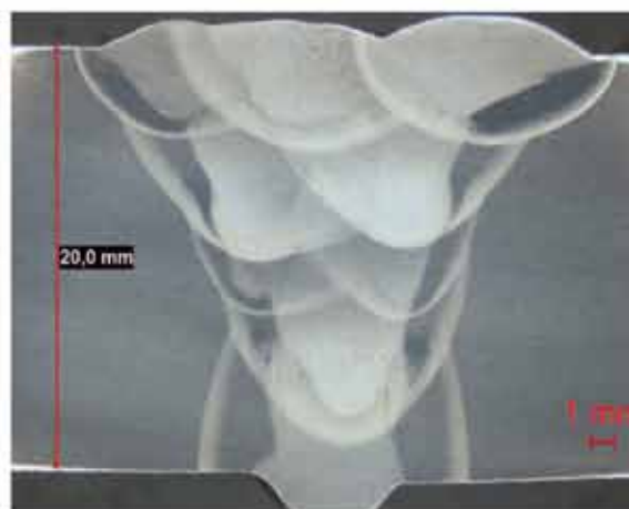
S355, butt joint, single-V butt weld with 30° included angle, on ceramic backing bar
